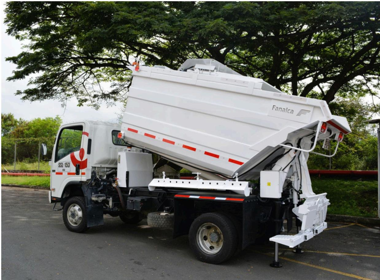
Rear-loading equipment for hard-to-reach areas, assisted by a lifter and bagging basket. Designed for transfer to other rear-loading equipment with a hopper or for disposal at final disposal sites. High operational efficiency and leachate containment.
